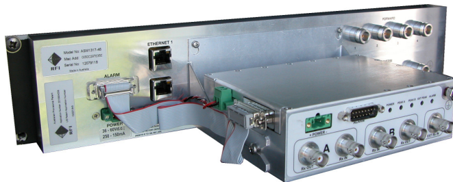
RSM FITTED TO ANTENNA SYSTEM MONITOR
